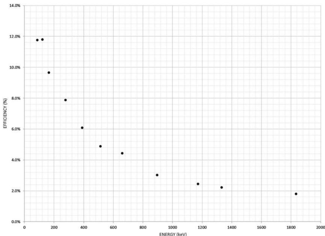
Fig. 2. Energy calibration curve for Colorado State University's HPGe detector system.
