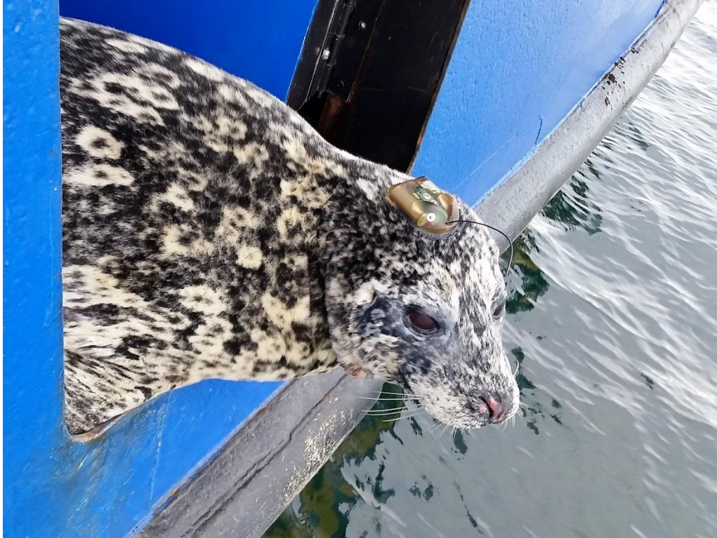
Figure 2. Splash satellite tag attached to the head of an adult male harbor seal.
