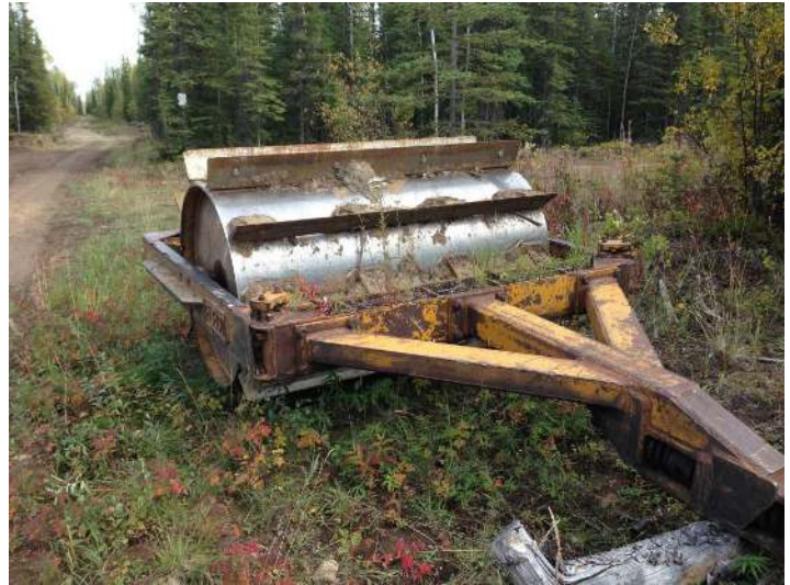
A roller chopper: 140 acres of land near Tok was treated with the roller chopper in the summer of 2015. Fish and Game, the Alaska Division of Forestry, and the Ruffed Grouse Society are working together to use this technique to enhance habitat on as much as 2,000 acres in the Tok area over the next four years
